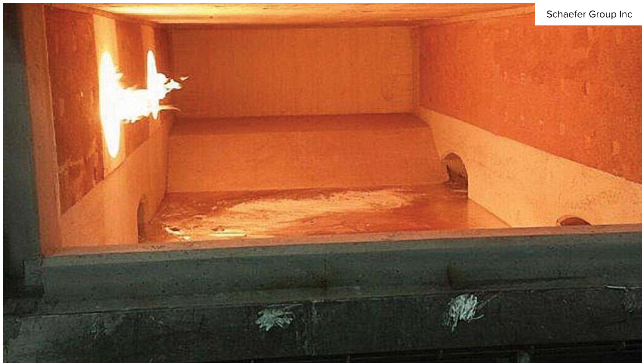
A high-headroom central melter with a preheated hearth.
