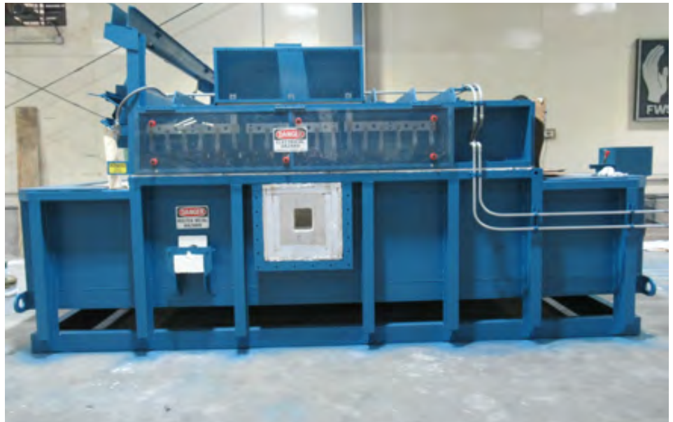
Electric "in cell" melter
